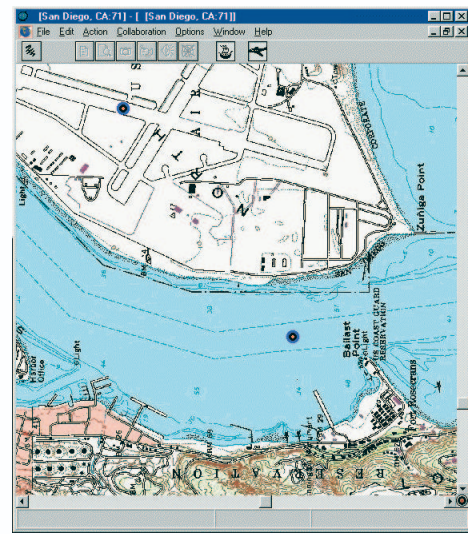
Figure 2. Multimodal Map. Objects tracked in a video are simultaneously displayed on a geo-referenced map.
